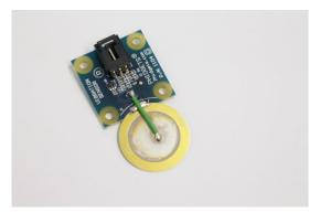
A device that uses the piezoelectric effect to measure changes in pressure, acceleration, temperature or force.
